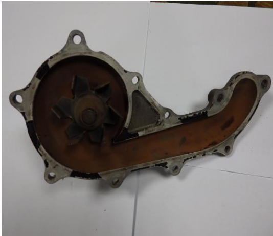
Corrosion of coolant
