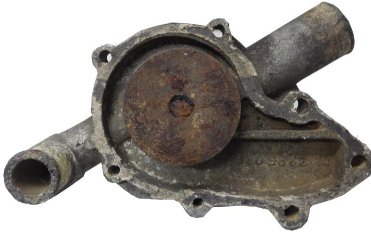
Coolant degradation / Corrosion
