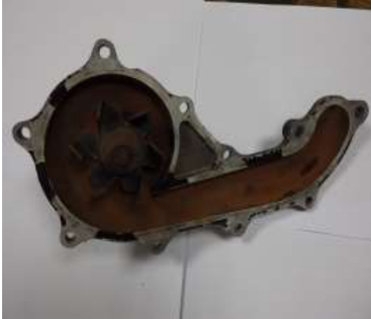
Corrosion of coolant
