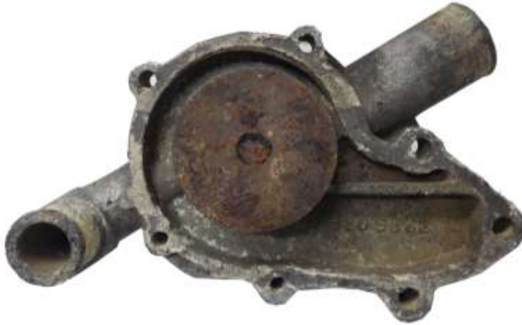
Coolant degradation / Corrosion
